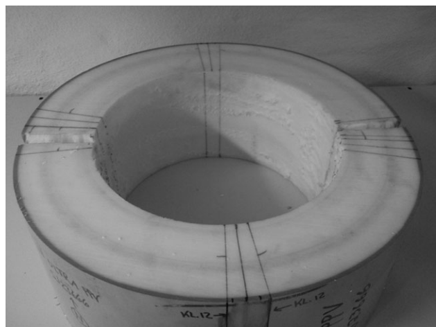
Figure 1. A section of polymer pipe insulation removed from the pipe. Total thickness of the insulation is 80 mm of which two layers with a total thickness of 64 mm are high-density foam.
